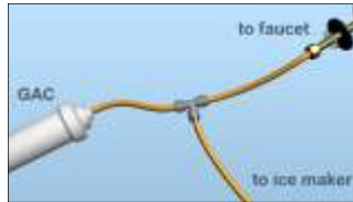
Figure 15. Connect the Ice Maker as shown (color of tubing is for illustrative purposes)
