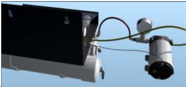
Fig. D7: Connect pump to pump jack on main frame
