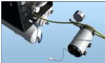
Fig. D5: Insert yellow tubing from the feed assembly to pressure gauge
