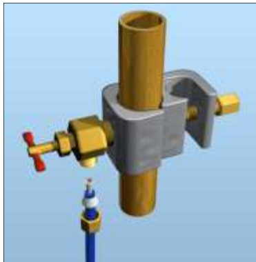
Figure 9. Connect tubing as shown (color coding of tubing is for installation purposes)
