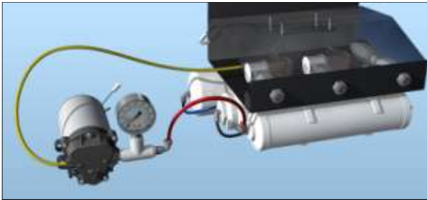
Fig. D6: Connect red tubing from pump outlet to CARB 12 inlet
