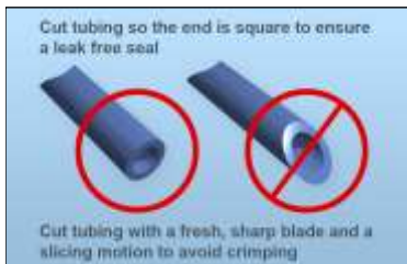
Figure 10. Cut tubing square; do not use scissors
